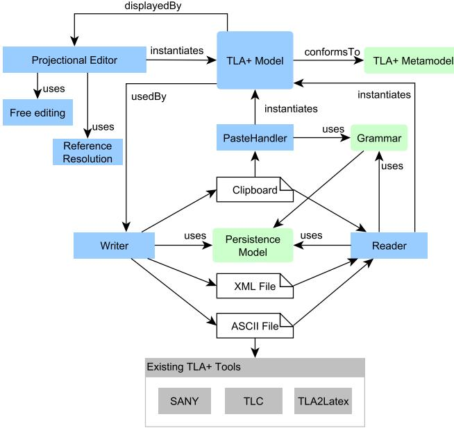
Fig. 1. Underlying architecture of SpecEdit
